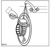
The dishwasher must not be used without filters. Incorrect repositioning and fitting of the filters will produce poor washing results. Cleaning the filters is vital to ensure correct operation of the machine.
